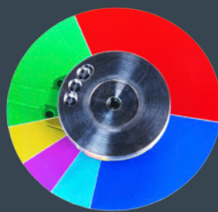
Top: Electron microscope image of a DMD chip showing the micromirrors in comparison to the tip of a pin. Above: RGBCMY 'Brilliant Colour' colour wheel from a single chip projector.
